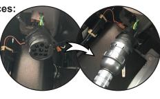
**OBD Devices:** Connect the OBD extension cord to the device, then plug
